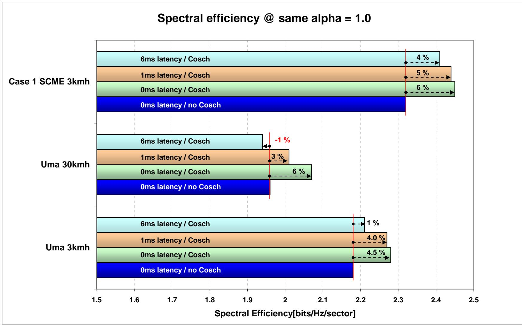
Spectral Efficiency = f(latency) @ same cell edge throughput
