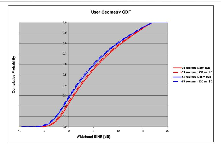
User Geometry = E[S]/(E[I] + R\*N) S = Signal Level, I = Interference Level, R = Receiver Noise Figure
