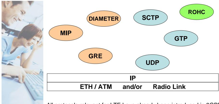
All protocols relevant for LTE have already been introduced in 3GPP. Some (e.g. SCTP) are however used in a slightly different way.
