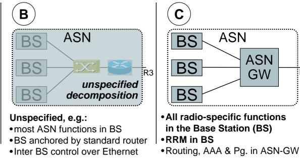
**Real deployments** may combine parts of different functional entities within on network element. Example: ASN-Gateway with incorporated CSN functionality:
